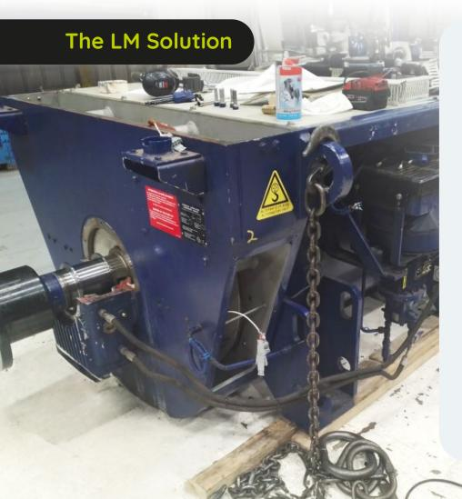
Although the generator was not directly at fault, the LM team identified overheating in the exciter rotor after electrical testing. Our failure report concluded:
